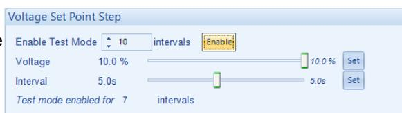
The voltage *Set Point* is increased and decreased by a pre-defined percentage, at the set interval for a set number of cycles. For commissioning the default values of 10 intervals, voltage steps of 10 % and interval delay of 5 seconds is used.
