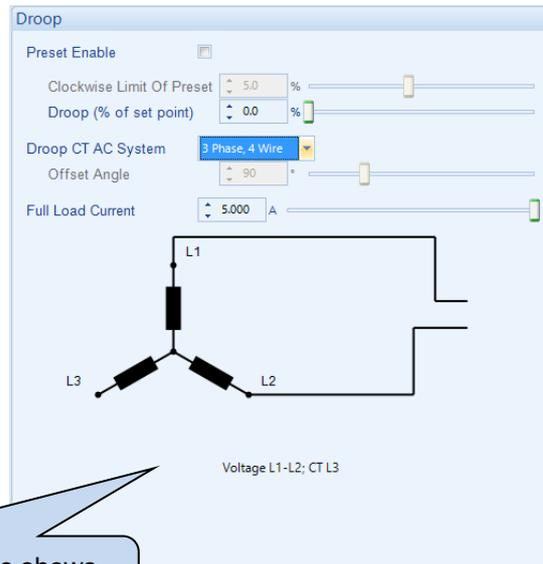
DSE Configuration Suite PC Software shows the location that the droop CT MUST be fitted.
