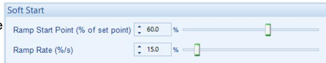
The *Ramp Start Point* value determines the percentage of the configured voltage *Set Point* at which the *Soft Start Ramp* takes effect. If a voltage spike at a value below the voltage *Set Point* is shown on start up, decrease this value. The settings should then be adjusted to allow for the smoothest start up in the optimum time for your application.
