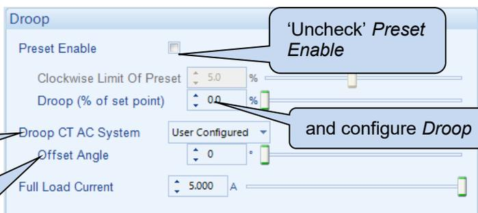
Set *Full Load Current* to match the CT secondary current when the generator is at full load.
