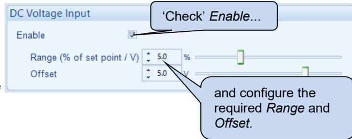
An open circuit input is treated as a 0 V input and so reduces the output voltage to the appropriate percentage of the set point. Using the above example, an open circuit input would reduce the output voltage to 207 V.
